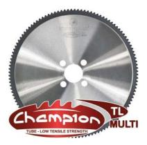
A dedicated Champion TL Multi saw blade has been developed for multiple tube cutting with a tensile strength of  $400 - 800 \text{ N/mm}^2$ . This blade type is specifically suited for Rattunde Twin machines but also for other applications where multiple tubes are being cut, such as the BEWO, RSA and Sinico machines.
